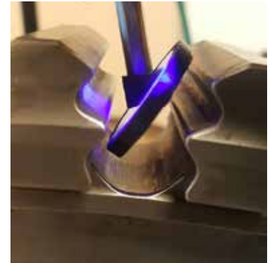
Add-on accessories enable access to sidewalls, inside grooves and bores.
