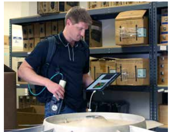
Portable inspection makes it possible to measure large components at the point of processing on the factory floor. The rolling workstation (left) and backpack/holster options (right) both facilitate shop floor inspection.
