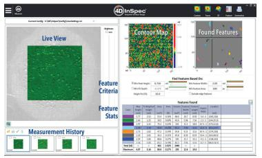
After pointing and clicking to take a measurement, operators easily verify the area they are measuring (left, live view area).
