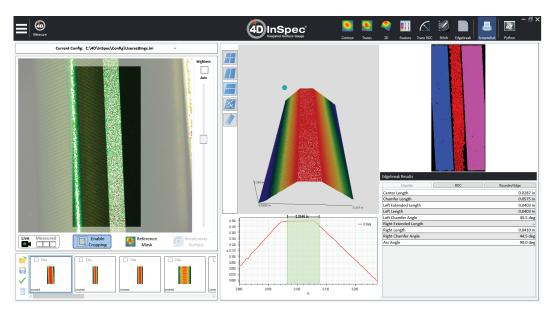
One of the difficulties of measuring edge break is the challenge of lining up the gauge system perpendicular to the edge. With 4D InSpec's area measurements, even if the 4D InSpec is cocked to the edge, the software calculates the surface planes from the data, and then measures the edge break surface (chamfer, rounding or radius). The improved time savings could amount to hours per shift, while the data is numerical and precise.
