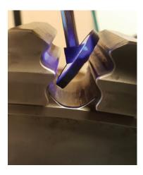
4D InSpec's many accessory options include a fold mirror kit, to help you measure sidewalls, inside grooves and holes—or deep inside a fir tree.
