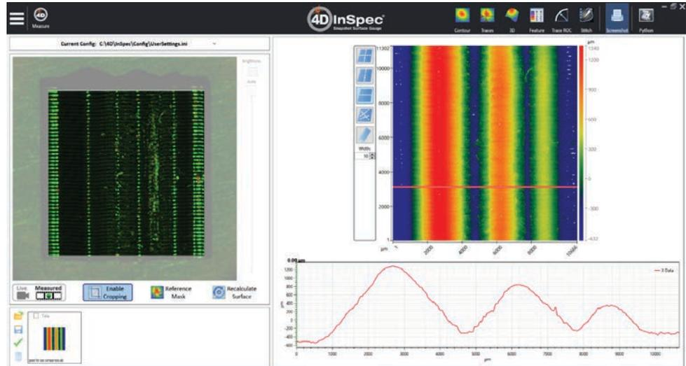
Figure 2: 3D Measurement (plotted, upper right) of sample part (green camera image on the left) using 4D InSpec XL. A 2D trace was drawn across one slice (red line, bottom right).
