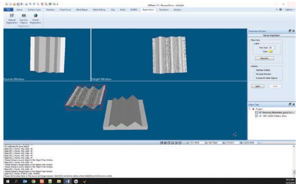
Figure 8. Initial placement of source and target in the alignment process.
