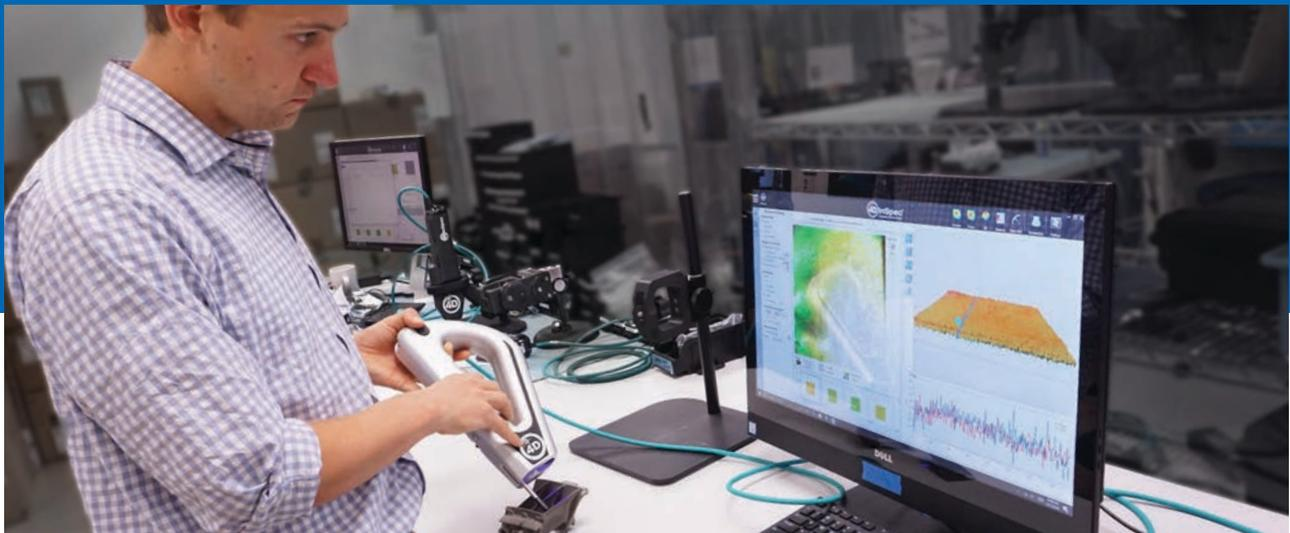
Hand-held 4D InSpec XL provides 3d surface defect measurements in seconds, complete with pass-fail analysis of the large 15 mm field of view. Rugged enough to use on the shop floor, yet precise and repeatable results make it a breakthrough for machined/additive parts manufacturing, QA and MRO.
