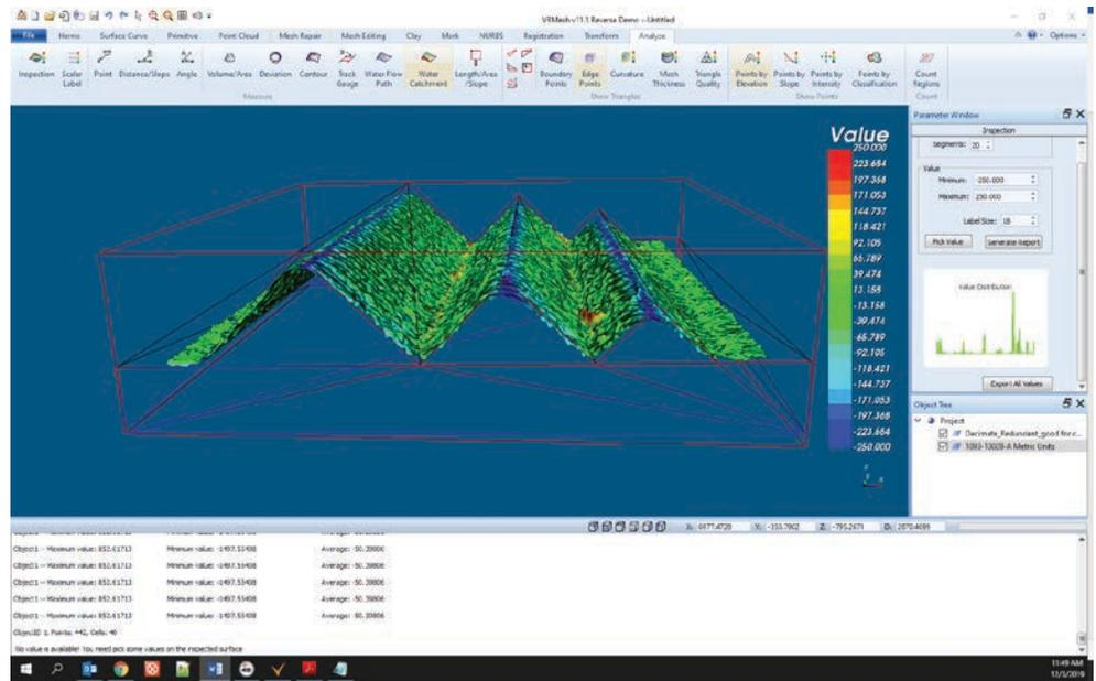
Figure 14. After adjusting height scale, differences in the model versus the part jump out as high spots (red) and low spots, (blue).
