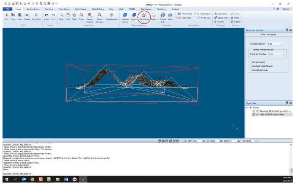
Figure 10. Turning on the wireframe display of the CAD model.
