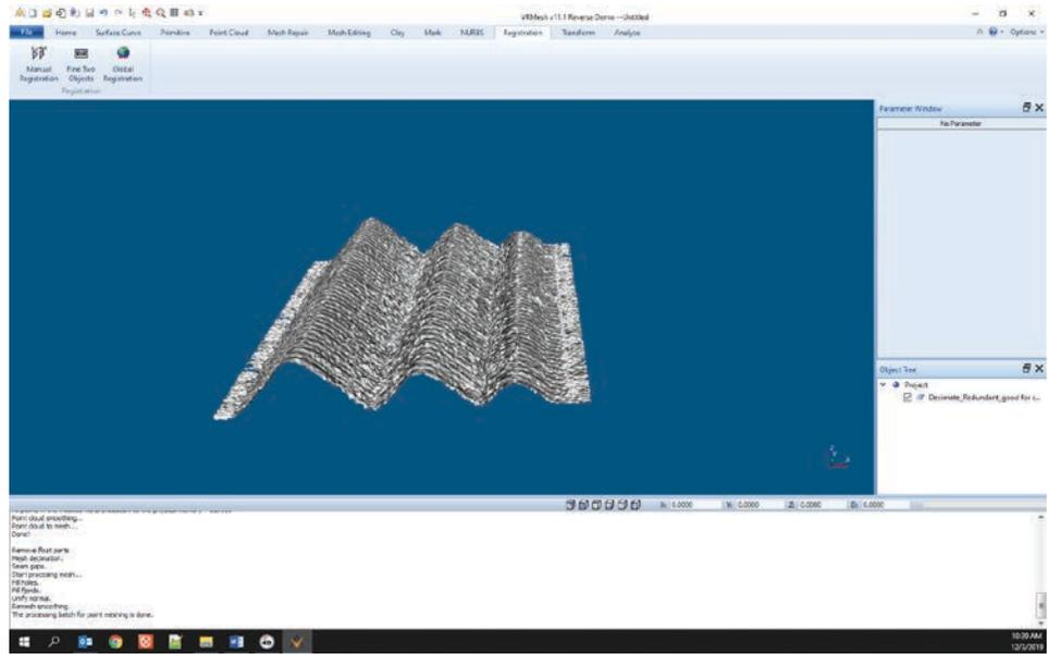
Figure 5. The mesh, after converting the point cloud to mesh.
