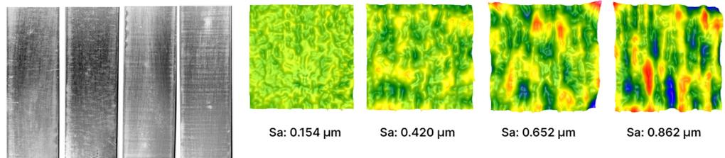
Figure 4: Four aluminum surfaces (left) appear similar in texture. However, filtering the 3D data into wavelength bands (right) reveals increasing degrees of roping. Results shown in Bandify3D software. Data and analysis courtesy General Motors.
