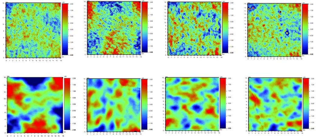
Figure 5: Four substrates (top) and final painted product (bottom). All measurements use the same false-color height scale.
