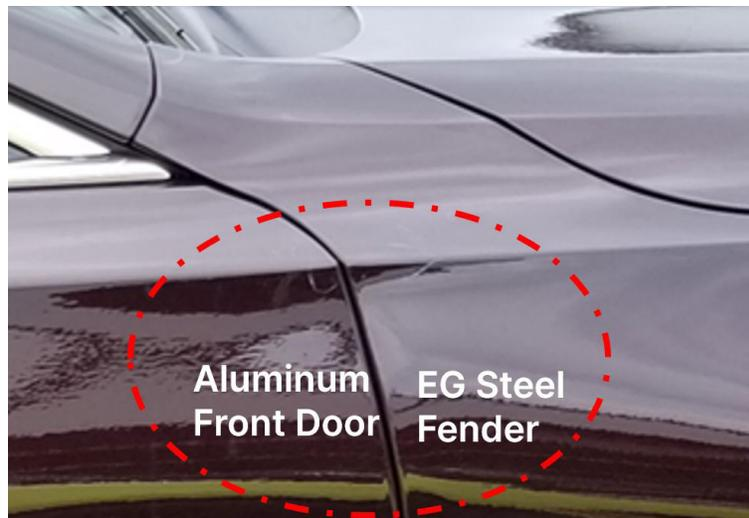
Figure 1. Current methods. An aluminum panel next to steel panel show clear texture differences. Courtesy of General Motors.
