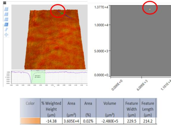
Figure 7: 3D surface measurement (upper left), identified pit (upper right), and quantification of depth, area, width, and volume of the pit (bottom)
