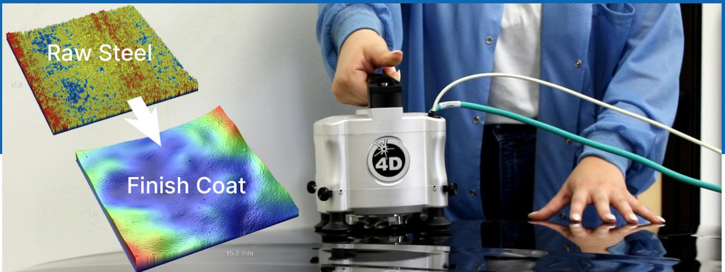
4D SurfSpec measures rough and smooth surfaces to fingerprint paint and coating processes.
