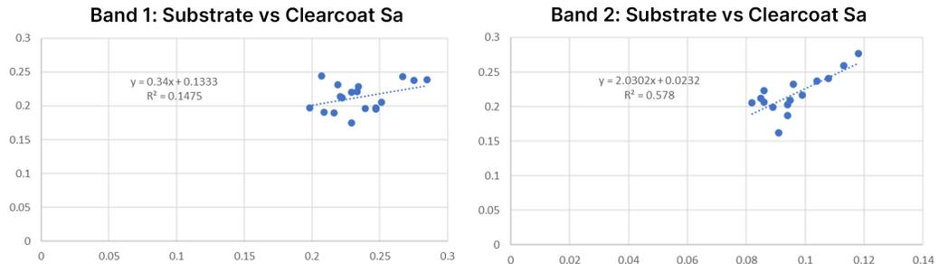
Figure 6: While analyzing one wavelength band does not differentiate this set of substrates (left), analyzing a different band shows a higher degree of correlation (right).
