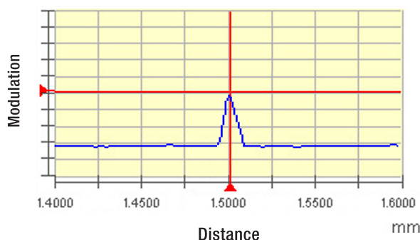
Figure 5. Path matching results for a transparent disk using the remote cavity method.
