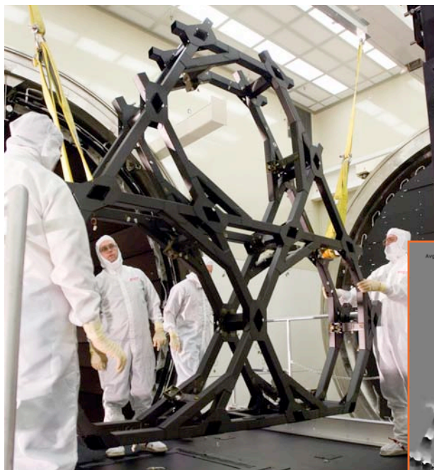
Figure 4a. The support structure for the James Webb Space Telescope undergoes cryogenic testing for dimensional stability. (Courtesy Northrop Grumman ATK Space Systems).
