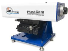
**PhaseCam®** dynamic Twyman-Green interferometers provide high resolution measurements in as little as  $1\mu\text{s}$ —5000 times faster than temporal phase-shifting interferometers. Compact and lightweight, PhaseCam systems make reconfiguring test setups simple and allow for in situ measurement and on-machine polishing metrology.
